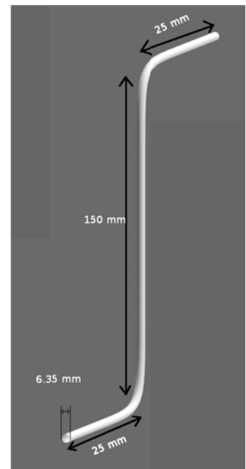
Illustration 8: Design of the gas sampling tube
