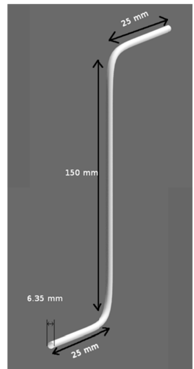
Illustration 5: Design of the Pitot tube
