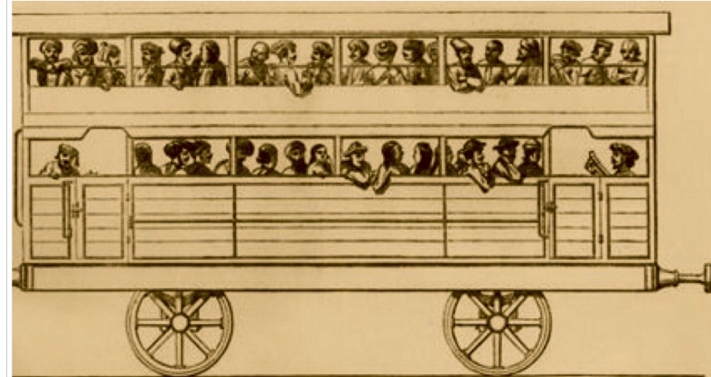
TWO-TIERED THIRD-CLASS CARRIAGE OF THE NORTON, BANHUA, AND CENTRAL INDIA RAILWAY.
