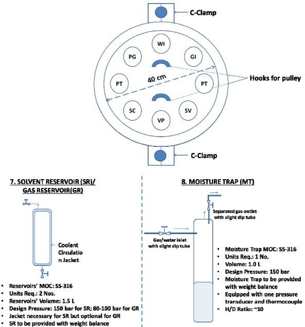
• Both reservoirs equipped with one pressure transducer and thermocouple each
