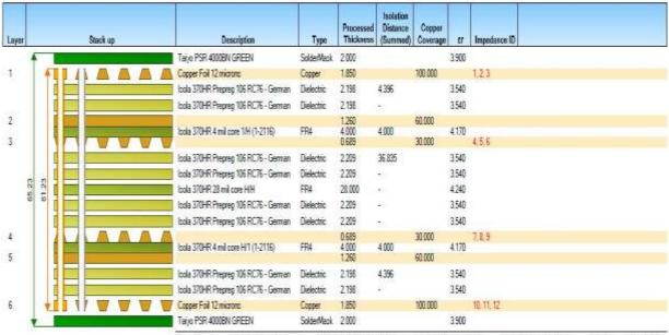
Coppor Thickness = 7.598 | Dielectric Thickness = 53.628 | Solder Mask Thickness = 4.000 | Stack Up Thickness = 61.226 | Stack Up Thickness with Soldermask = 65.226
