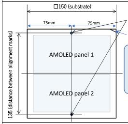
Alignment mark : φ0.6 (metal layer) circle shape Orientation Corner
