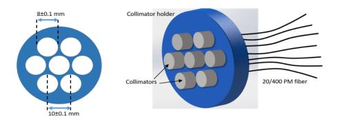
Individual collimators should have tip/tilt control
