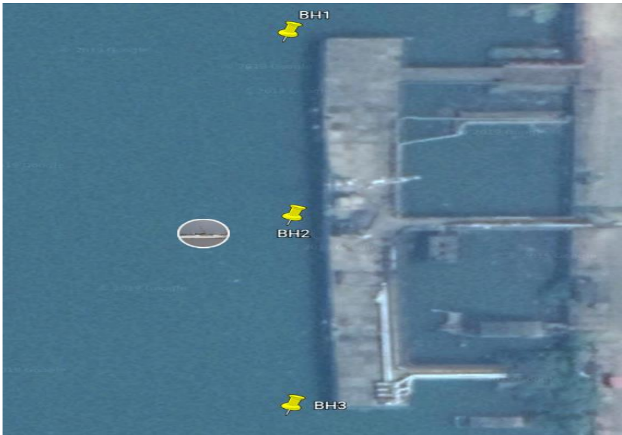
Fig 2. Tentative Bore hole location alongside South Coal Berth at Cochin Port Trust
