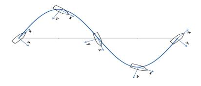
In pure sway mode of operation, the model is oscillated sinusoidally in the lateral direction with its axis always parallel to the axis of the towing tank. Here, both the struts move at the same phase.
