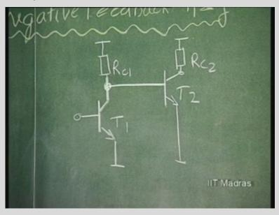
What is h? It is series at the input and shunt at the output. g feedback is shunt at the input and series at the output. h feedback is adopted in order to obtain a voltage control voltage source. So, h feedback is adopted for an idealization towards voltage control voltage source. g feedback for an idealization towards current control current source.
