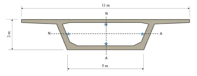
Figure 1: Cross section of the prestressed box girder bridge
