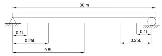
Figure 4: Layout of sections that would be instrumented.
